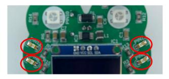
An LED, or **L**ight **E**mitting **D**iode, is an electronic component that emits light when an electrical current flows through it.
