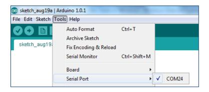
The last thing you need to do before you can write and upload a sketch is tell the IDE which type of board you are using. There are many different types of Arduino boards. The MC Trainer is based on the Leonardo, so select "Arduino Leonardo" under Tools > Boards.
