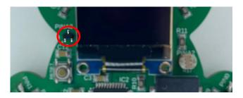
The temperature sensor on the MC Trainer is a linear active thermistor. These temperature sensors give out a voltage signal that changes directly with temperature. This means the relationship between the voltage output and the temperature is straight and direct, making the data easier to read and use.
