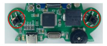
A button, also known as a push-button or momentary switch, is a simple device that allows a user to interact with a piece of machinery or electronic device. Buttons complete or break an electrical circuit when pressed, allowing for control of an electrical system.
