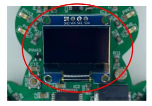
OLED stands for organic light emitting diode. This small screen allows for real-time feedback and interaction with projects.
