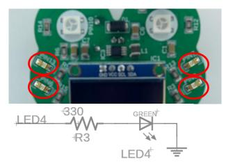
Four single LEDs are controlled by digital pins 8, 13, 6, and 7. There are four separate circuits, but they all do the same thing. Each LED is controlled by programming the pin on the 32U4 chip to enter a **HIGH** or **LOW** voltage state. The LED is turned on when the pin voltage is set to **HIGH**, which creates a difference in electrical potential between the pin and ground. This causes current to flow through the LED.
