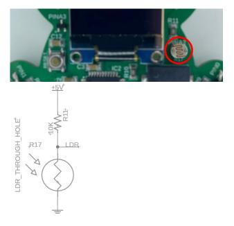
Analog pin A2 is connected to a light-dependent resistor (LDR), a component that varies its resistance in response to changes in light intensity striking its surface. This behavior of the LDR, sometimes referred to as photo resistivity, can be used as a gauge to measure and monitor ambient light conditions. As the resistance of the LDR fluctuates with light intensity, so does the voltage across it. By reading this voltage with analog pin A2, we can gain an insight into the ambient light level.
