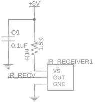
Digital pin 17 on our Arduino Leonardo is connected to an infrared (IR) receiver. The IR receiver is a specialized electronic component designed to sense infrared light which falls beyond the range of human vision. This IR receiver detects infrared signals, transforms them into electrical signals, and forwards them to the MC Trainer. When an IR signal is detected, it influences the output voltage of the receiver.
