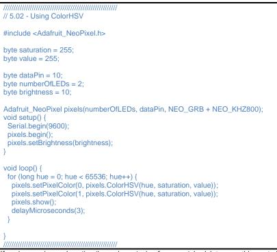
\*If you're copying and pasting the code, or typing from scratch, delete everything out of a new Arduino sketch and paste / type in the above text.
