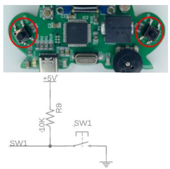
The MC Trainer has two momentary push buttons. SW1 is on the left side of the board and is measured by digital pin 1, and SW2 is on the right and measured by pin 0. The switches are normally open. A 10K resistor acts as a "pull up," which weakly pulls each pin to 5V so that they consistently will read a digital **HIGH** when the switch is open. Pushing the switch moves the pin to digital **LOW**.
