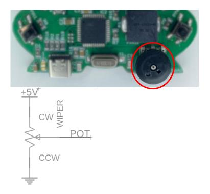
Analog pin A0 on our microcontroller is interfaced with a potentiometer, a type of resistor that allows for adjustable resistance. The unique characteristic of a potentiometer is that its resistance varies as you turn its knob or slide its lever. As the resistance of the potentiometer changes, the voltage observed at pin A0 also adjusts. This change in voltage can be measured and interpreted by the microcontroller to understand the current setting of the potentiometer.
