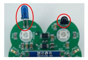
An infrared emitter and detector are paired electronic devices that enable wireless communication and sensing applications using infrared light. These components are found in a wide range of devices, including remote controls, security systems, and obstacle detection systems for robotics.
