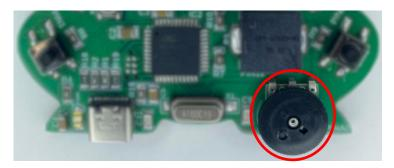
A potentiometer, often referred to as a "pot," is a type of variable resistor. They are commonly used for controlling electrical devices such as volume controls on audio equipment or as control inputs in many types of electronic circuits. It's a three-terminal device that operates as an adjustable voltage divider.
