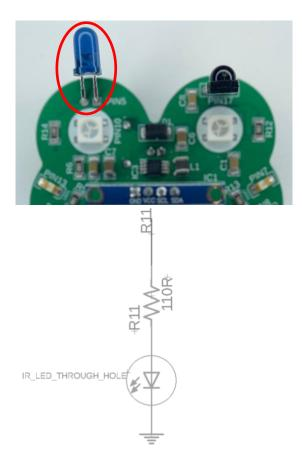
Digital pin 5 on our microcontroller is connected to an infrared (IR) LED. An IR LED, similar to a normal LED, emits light when it is energized. However, unlike a regular LED, the light emitted from an IR LED is invisible to the naked eye as it falls within the infrared spectrum. When digital pin 5 sends a HIGH signal to the IR LED, it turns on and emits infrared light. Conversely, when the pin sends a LOW signal, the IR LED turns off and stops emitting light.
